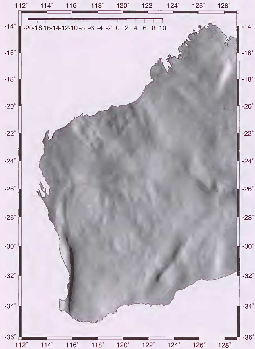
Figure 3. Computed AUSGeoid98 east-west vertical deviations across Western Australia (Mercator projection; Units in arc-seconds).
